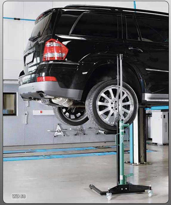
Compac's wheel lifter is an ergonomic solution for easy and safe demounting, handling and mounting of aluminium wheels with low profile tyres up to 24".
