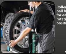
Rollers with ball bearings for easy rotation and positioning.
