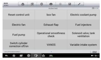
Figure 4-16 Sample Active Test Screen
