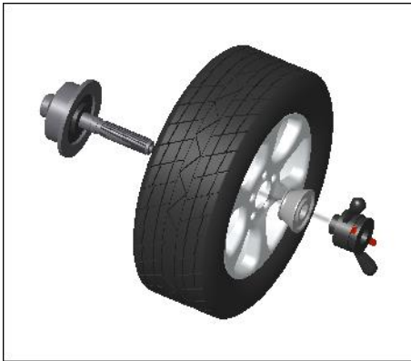
Main shaft—wheel –cone—quick lock nut
