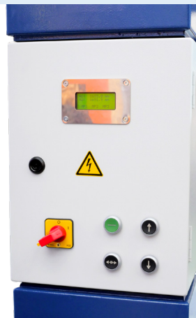
The HDL 6500, HDL 7000 and HDL 8000 offer 2 control units, one on each side
